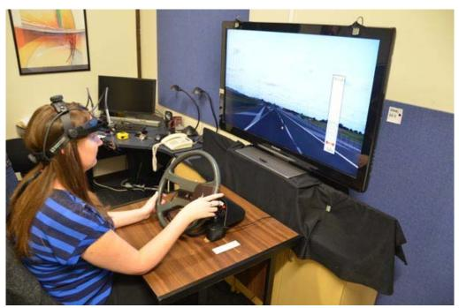
Figure 11. The TARS eye-tracking equipment recording a participant's eye movements while viewing a road scene.
