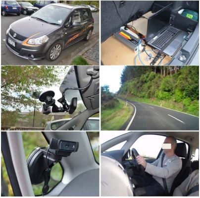
Figure 19. The car, computer system, video cameras and screen shots (from the video cameras) from the naturalistic driving testing.
